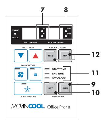
Temperature Scale LED Illuminates to indicate the current temperatures being displayed are either in °C or °F; also displays the clock when programming.
